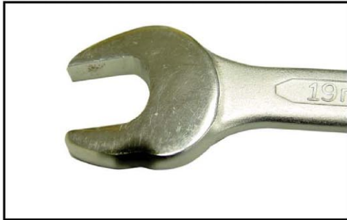
Electrical Burn Marks
