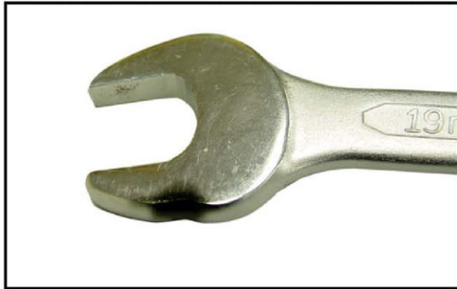
Electrical Burn Marks
